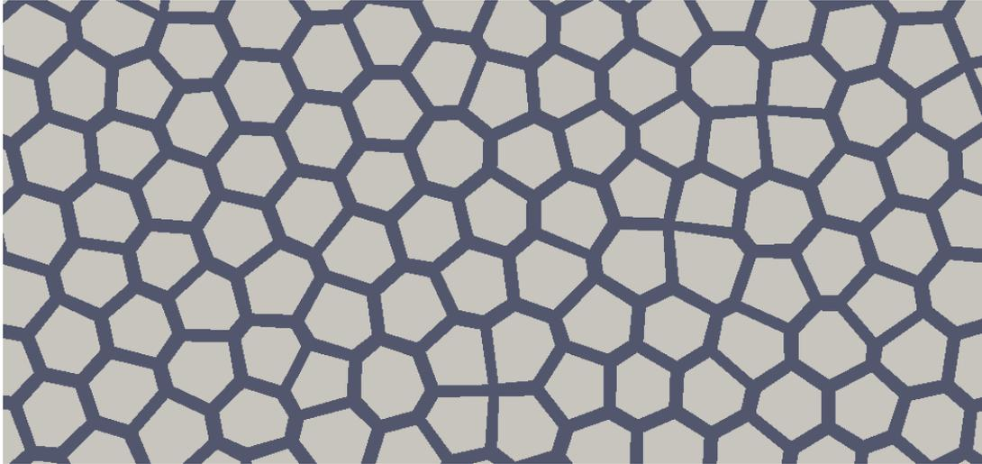
Figure 3.4.: Visualization of a granular medium with approximately equally sized magnetic grains (here: 4 nm diameter) surrounded by nonmagnetic material separating neighboring grains by 1 nm.
