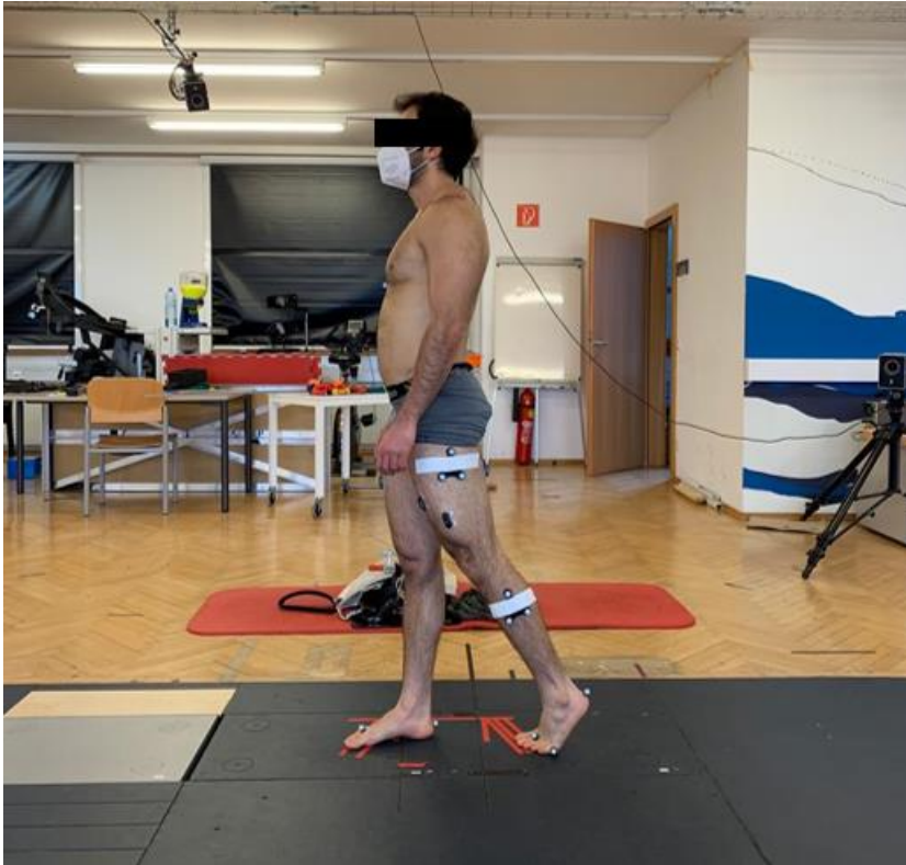
Figure 10: Example of a participant performing a gait trial while appropriately impacting the force plates with the left and right foot.
