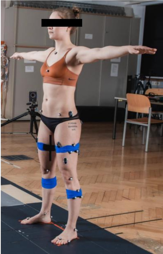
Figure 9: Example of a participant fitted with all 21 retroreflective surface markers, five tri-lateral marker clusters and a wireless EMG electrode, assuming the static T-pose.
