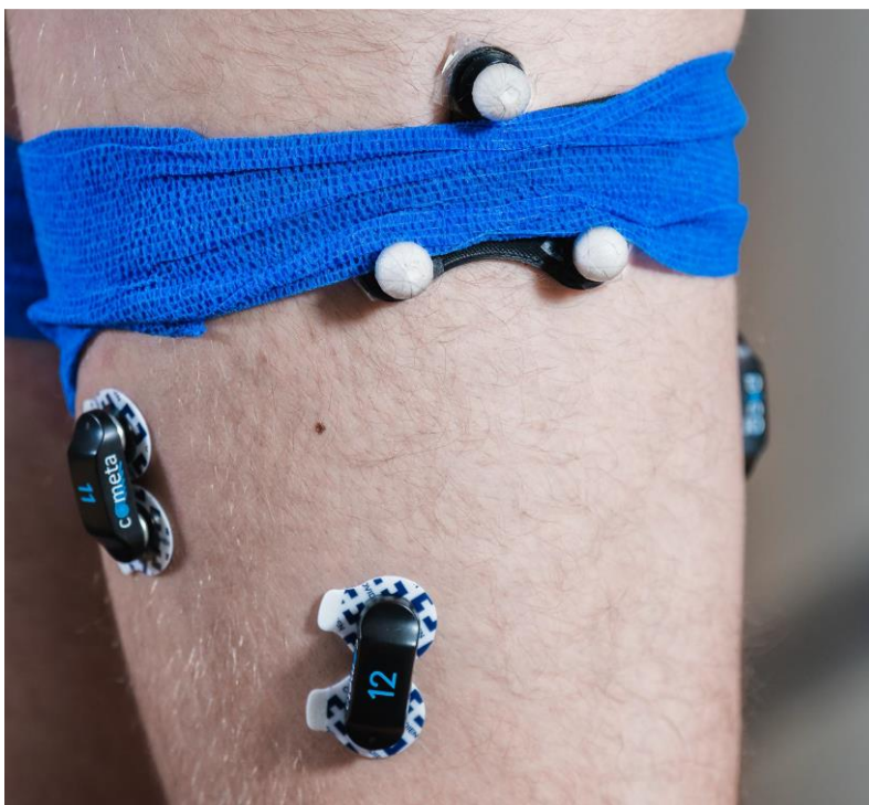
Figure 13: Example of a trilateral marker cluster and its fixture method
