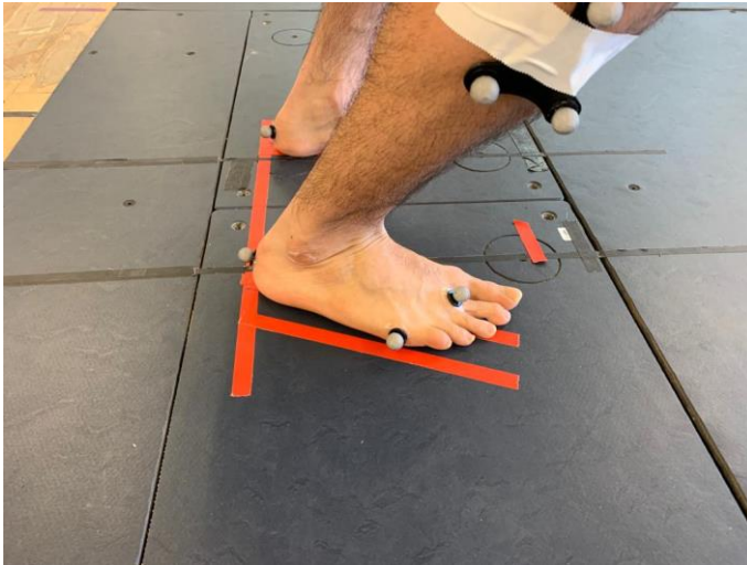
Figure 11: Floor markings on the force plates used to standardize foot positioning in regards to foot angle and stance width
