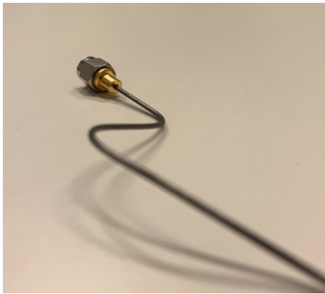
Figure 4.14.: A superconducting coaxial cable inserted into the SMA crimp connector.
