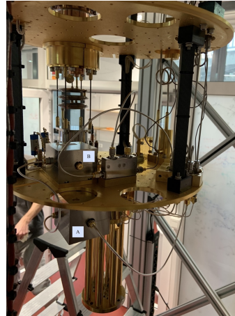
Figure 4.10.: A front view of the installed circulators
