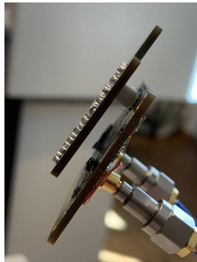
Figure 3.17.: PCB v3 from the side, with the filter PCB attached while being measured on tabletop.
