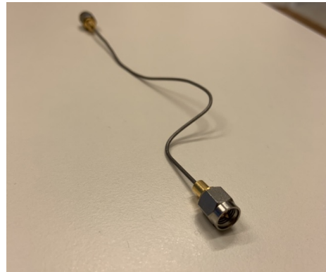
Figure 4.15.: The superconducting coaxial cable with 'S' shapes formed.
