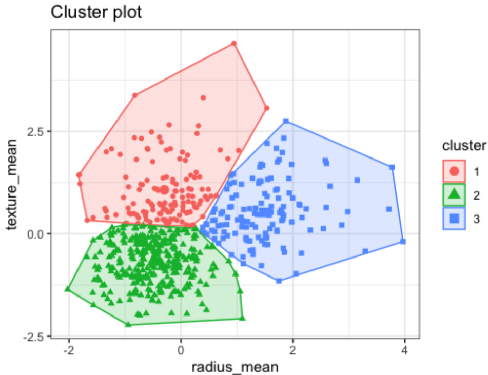
Figure 3.1 – Three clusters as an outcome of the k-means algorithm run with k=3 . The separation was based on two variables: texture and radius (Illustration from Harezlak, 2022).
