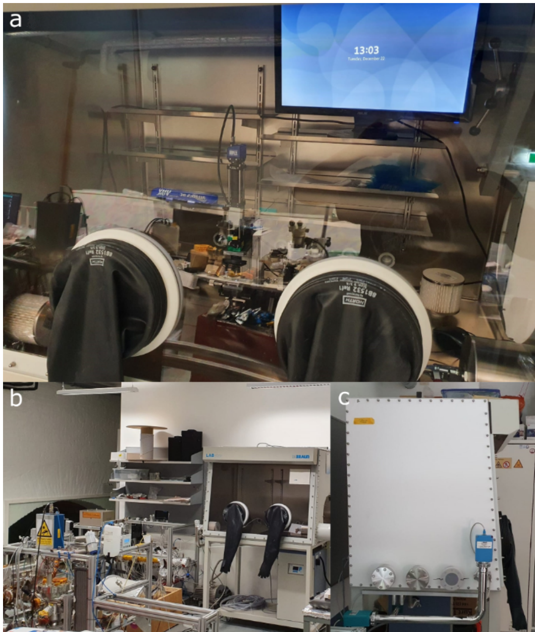
Figure 3.9: Photographs of the glovebox at Sternwarte laboratory. Image a) shows the inside. The microscope setup, a computer with screen, mouse and keyboard, the heating stage as well as power supplies, the vacuum tweezer and sample storages are visible. Image b) shows the glovebox next to the loadlock part of the CANVAS system, the loadlock in the front and the up-stairs sample "garage" in the back. Image c) shows the custom made sidewall with the three ports. The port on the right side can be connected with the loadlock. The blue boxes connected to the steel pipe are the detectors of the gas cleaning system. Photo courtesy by Felix Herterich.
