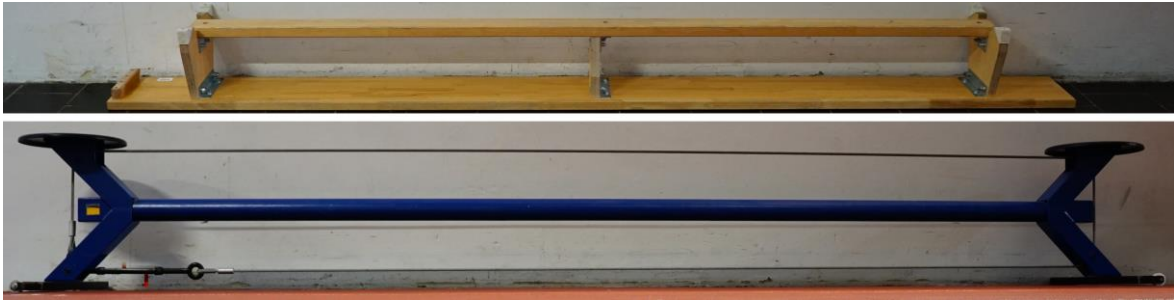
Figure 1: Top image shows the upside-down gymnastics bench which was used for BEAM conditions. Bottom image shows the THIGHTROPE mounted on a rack between two platforms.
