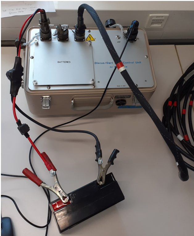
Figure 5: The control unit which provides power to, and controls the DART probe.
