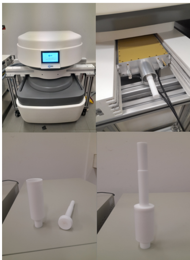
Figure 7: Clockwise from top left: rock analyzer used for lab NMR from the company 'Niumag corporation' based in China, core holder, sample holder sealed and unsealed with a lid which is where the sample is placed into.
