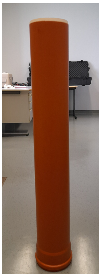
Figure 31: The pipe used to demonstrate borehole conditions with dimensions: height= 1.120 \pm 0.001 m and diameter 0.151 \pm 0.001 m.
