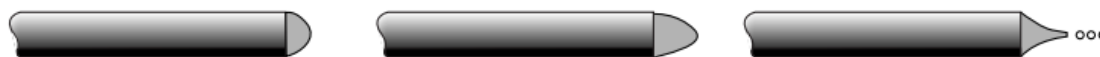
Figure 13: Representation of the conformation of the droplet into a Taylor cone (Hoffmann and Stroobant, 2007 p45).
