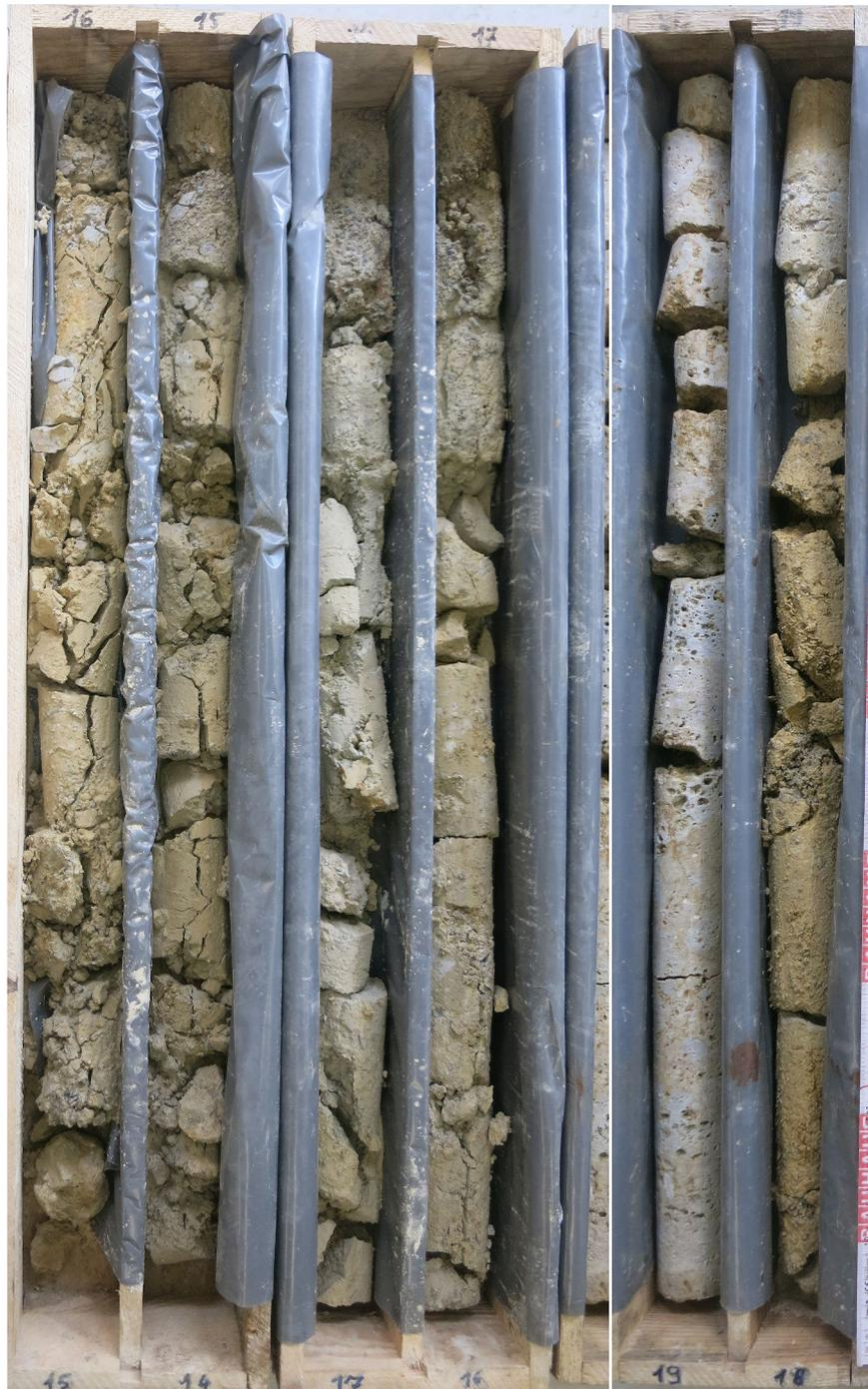
**Figure B.1** – Drillcores m14-20. The samples are relatively wet, ochre coloured and heavily fractured. One can see tectonic breccias as well as "cellular breccias" (m19-20).
