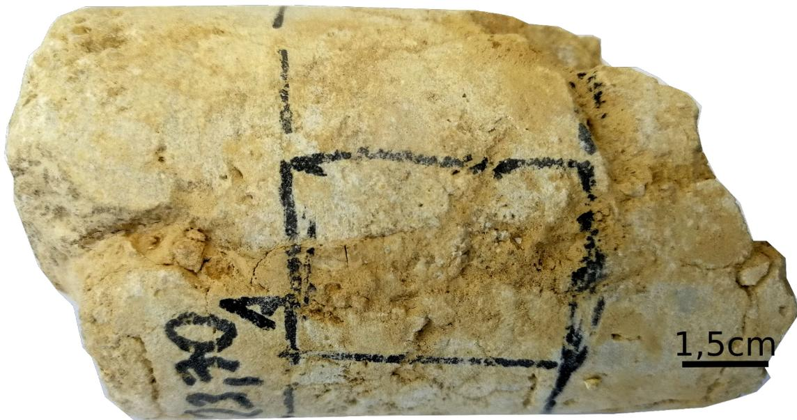
**Figure 4.37** – SFK1m23-70. The author paid attention to select a part of the sample containing matrix as well as breccia clasts. The sample is incohesive and the matrix weak. It contains slickensides which are not resolvable on the photograph.
