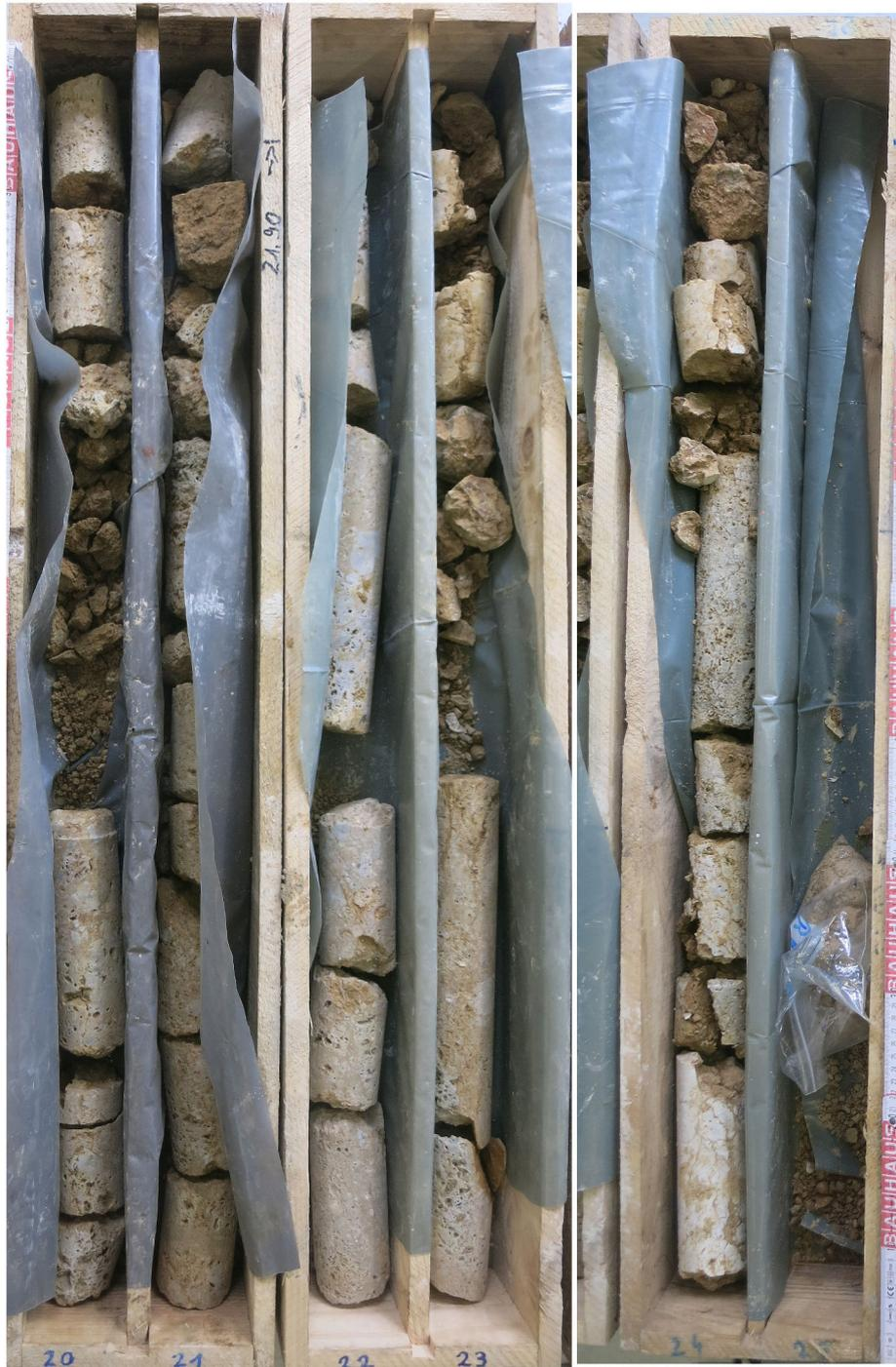
**Figure B.2** – Drillcores m20-26. Of great interest were the cellular breccias. The rocks are intensely weathered and show many open cells. Denser parts were referred to as carbonatic fault breccia. From m24-25, one can see a fracture containing fine-grained matrix and carbonatic clasts.
