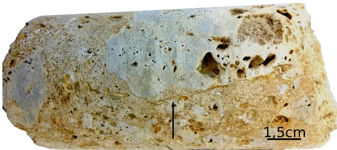
**Figure 4.12** – SFK1m20-40A. Clasts in the matrix range between mm-dm in size. Cells in the greyish-blueish components are rounded and chaotically arranged. Cell-diameters range from few mm to  $> 1.5$  cm. Towards the matrix, clasts are bordered by thin pressure solution seams (black arrow). Even though the sample is heavily weathered, it is cohesive.
