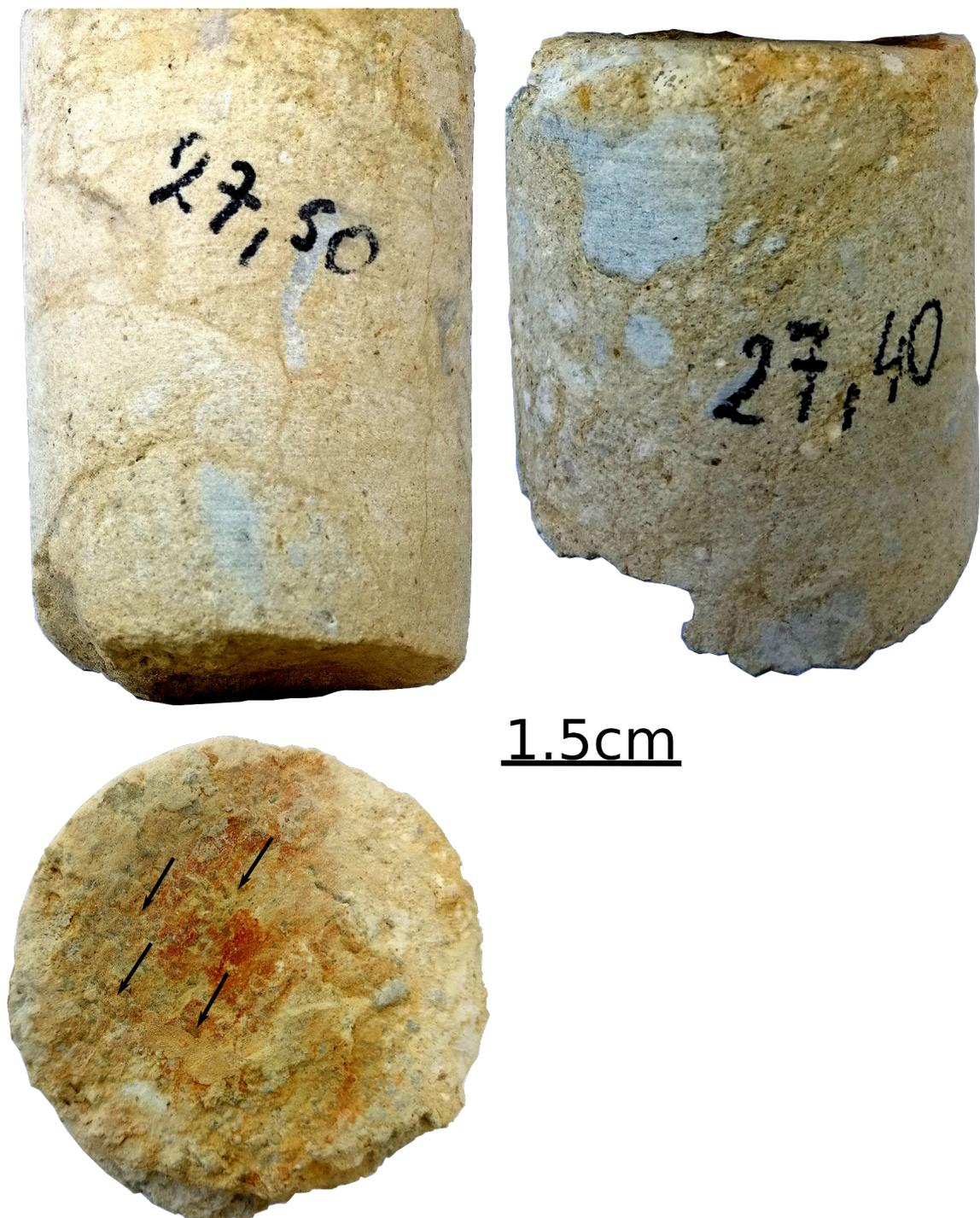
**Figure 4.42** – SFK1m27-40 and SFK1m27-50. Sutured, greyish carbonatic clasts in a intensely weathered matrix. Arrows tracing the orientation of reddish, metallic appearing slickensides. Unidentifiable lithic fragments are visible.
