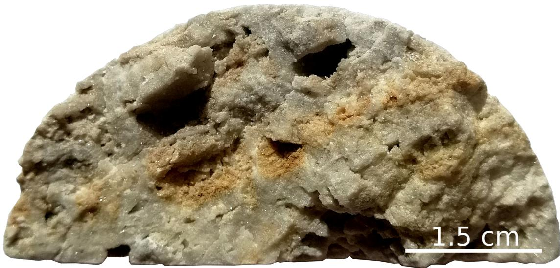
**Figure 4.24** – SFK1m19-50. Dissolved dol creates cells with uneven walls, encrusted with cc-crystals. Brownish spots derive from weathering and pressure solution.
