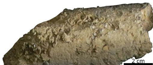
**Figure 4.29** – Hand specimen. Angular dolomite clasts in an ochre-coloured matrix.
