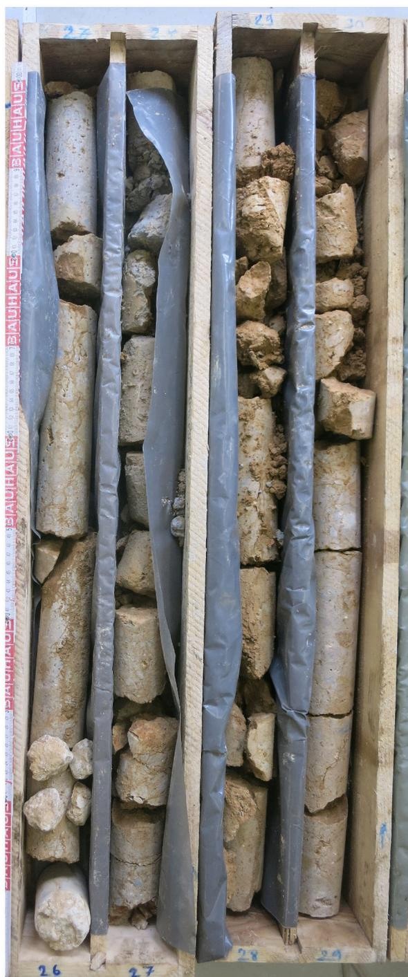
**Figure B.3** – Drillcores m26-30. Pressure solution overprinted the shapes of former fault breccia clasts (m26-27). In the cavern plan, these rocks are referred to as dolostone, dolostone-marble and dolostone breccia. Microscopic analysis revealed, that the main mass of the rocks indeed is calcite, with only little amounts of dol rock-flour as constituents.
