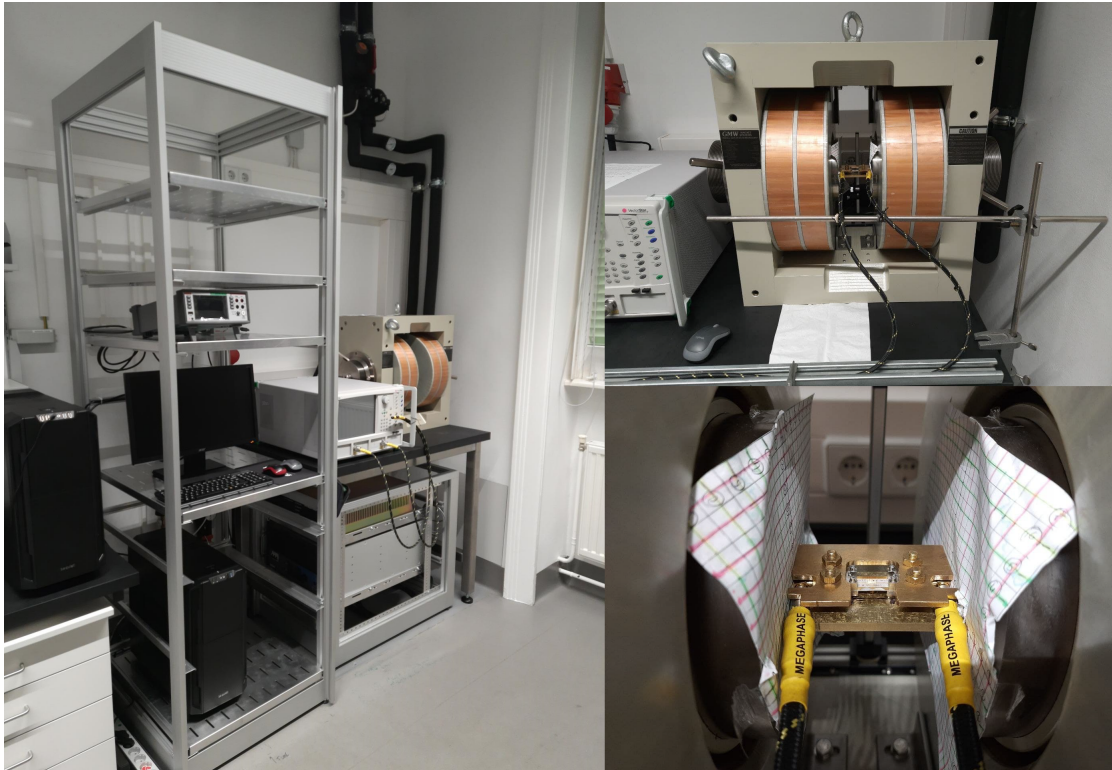
Figure 2.4: Pictures of the FMR laboratory. (l.) The FMR workspace, including electromagnet, power supply, source meter, VNA, and computer. (u.r.) A close-up of the electromagnet and the magnetic transducer. (l.r.) A close-up of the sample holder, microstrip, and sample.
