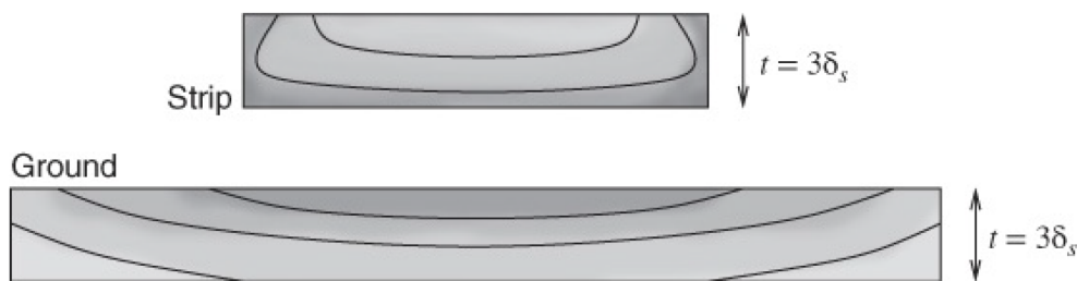
Figure 3.1: Transverse current density shown in the cross section of the strip and ground plane of a microstrip. Dark shading indicates higher current density. Taken from [4].
