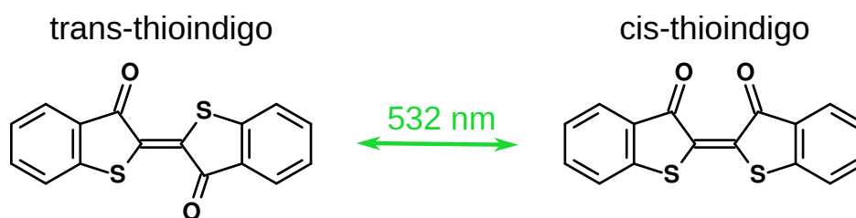
Figure 8.2: Photoisomerization of thioindigo C_{16}H_8O_2S_2 . The absorption of green light can change trans-thioindigo into the cis-isomer and vice versa. Both isomers absorb photons at \lambda \sim 532 nm. While the trans-isomer is fluorescent, the cis-isomer is not [278, 280].
