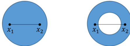
Figure 2-3 Convex (left) and nonconvex (right) sets. The two dots and line segments between them illustrate how to tell convexity of sets geometrically; A set C is convex if a line segment connecting any two points in C lies in C as well, otherwise, nonconvex.
