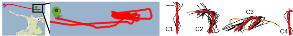
(a) GPS record, starting at the green marker and ending at purple. The zoomed area (right) shows the ship at dredging. (b) Cluster means (red) and char. segments (black) of the trajectory. One single right turn (orange dashed) in C3.
