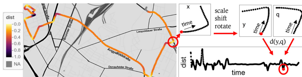
Fig. 1 GPS trajectory of a car driving eastwards, color coded according to the shift-scale-rotation-invariant distance to the query pattern q which represents a sharp left turn
