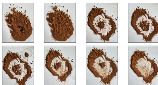
Figure 8. Photographs of the sampling procedure for evaluating the presence of CB in 250 g of solid contaminated with pigment paste. For more details, see the text.
