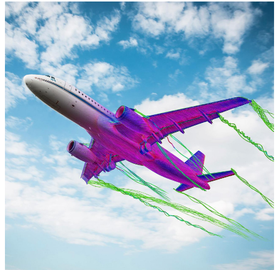
Fig. 1: CODA is a Computational Fluid Dynamics (CFD) solver for the simulation of aircraft aerodynamics and was developed in a joint effort between the German Aerospace Center (DLR), the French Aerospace Lab (ONERA), and Airbus. Copyright: DLR (CC-BY 3.0) [3].
