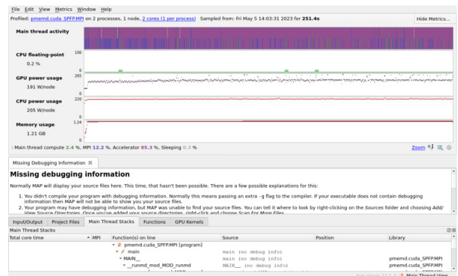
Fig. 2: Example profile involving the energy metrics optionally included in LINARO/FORGE/MAP ( https://www.linaroforge.com/linaroMap ).
