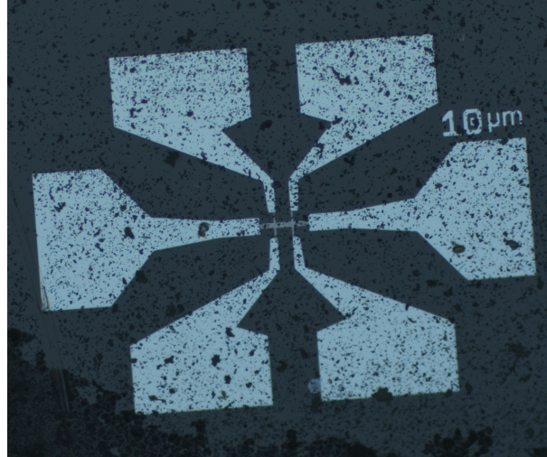
Figure 2.2: Microscope image of the structure on sample 230808 . The label of 10\ \mu\text{m} on the right side indicates its bridge width. What can clearly be seen and will be discussed in section 2.3 are residual areas of wax on the sample.
