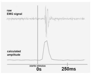
Figure 1. Electromyography: This figure shows the transfer from a raw EMG signal into an amplitude signal. Amplitude peaks which reflect eye blink magnitude were subject to statistical analysis.
