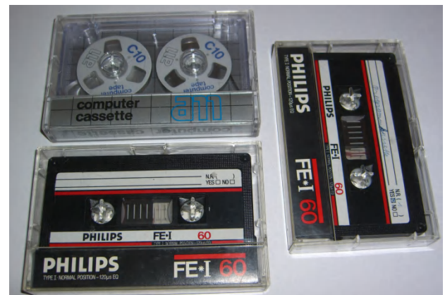
Figure 5: Tapes used for evaluation of migration tool, left upper corner C10 computer cassette, left lower and right Philips FE-I 60 normal position audio tapes.
