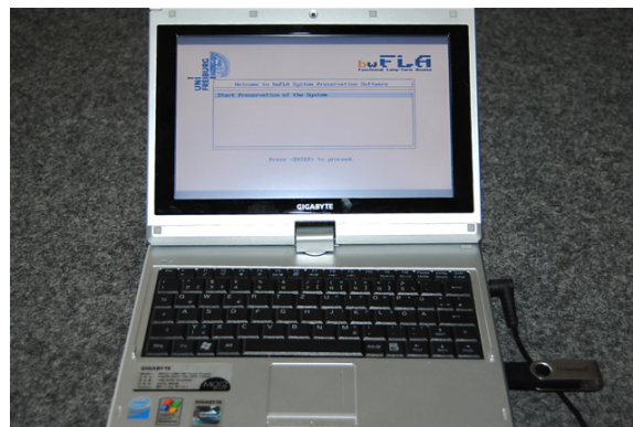
Figure 1: Target system booted from USB pen drive starting the system preservation process.
