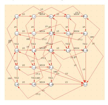
Figure 4: Our Markov modeling for a four-copy system (2 in disk and 2 in tape)
