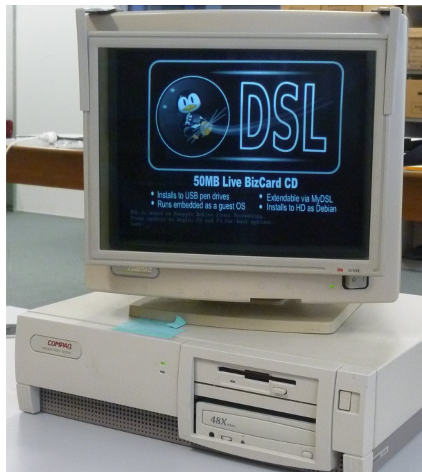
Figure 3: Booting Damn Small Linux on an x86 Compaq desktop machine to allow non-intrusive disk dumping
