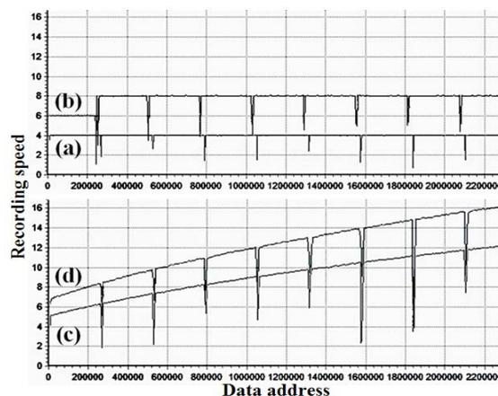
**Figure 1. Various recording conditions at (1)4x: CLV, (2)8x: zone-CLV, (3)12x: low speed CAV, (4)16x: high speed CAV.**
