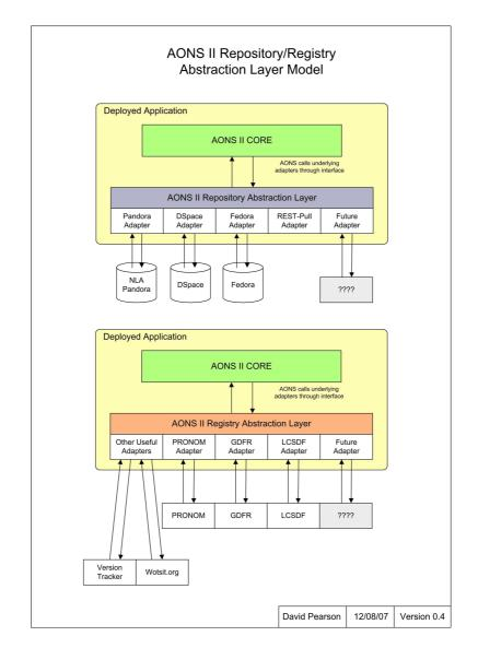
Fig. 2 Diagram showing the Repository/Registry Abstraction Layer Model. This diagram illustrates that the AONS II core code is separated from the various adapters so that the basic business logic does not need to be modified when creating or modifying adapters (*the author*).
