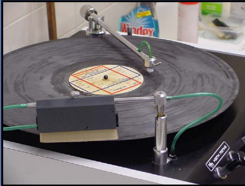
Transcription disk on Keith Monks cleaning device M/B/RS lab, Library of Congress
