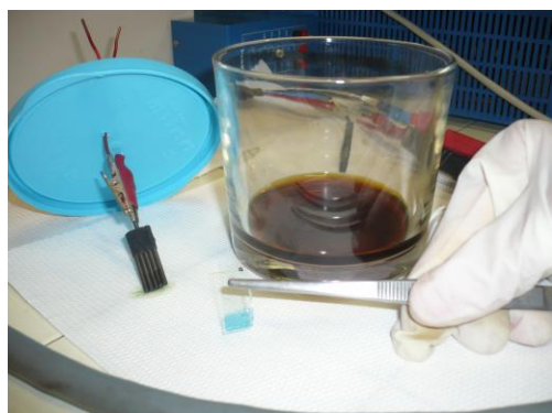
Figure 12. The working electrode after the electrochemical synthesis. (Image credit: L. Filippini, iNANO, Aarhus University, Creative Commons Share Alike Non-Commercial 3.0).
