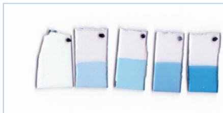
Figure 6. Four samples of Prussian Blue thin films, grown electrochemically over an ITO glass. First on the left is a piece of ITO with no film deposited. (Image credit: L. Filippini, iNANO, Aarhus University, Creative Commons Share Alike Non-Commercial 3.0)
