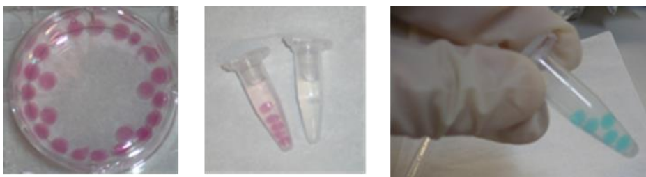
Figure 3 (Left): Calcium alginate beads with a red food dye entrapped; (middle): Red calcium alginate beads in water after overnight immersion; (right): Calcium alginate beads with a blue food dye entrapped. Image credit: L. Filippini, iNANO, Aarhus University, Creative Commons Share Alike Non-Commercial 3.0.
