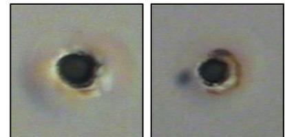
**Figure 10: Marks made in our recording layer on 1/2-inch tape, using less than 10 mW of optical power.**
