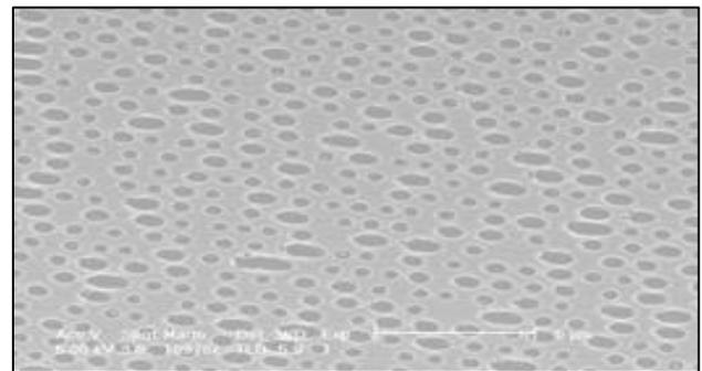
**Figure 3: Marks made on the M-Disc, as seen with an SEM.**
