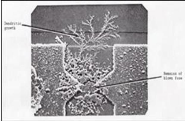
**Figure 8: A dendrite has grown from the remains of a programmed cell (blown fuse) in a PROM storage device.<sup>14</sup>**
