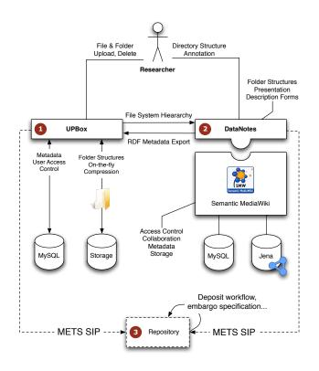
Figure 1: Architecture of UPBox and DataNotes
