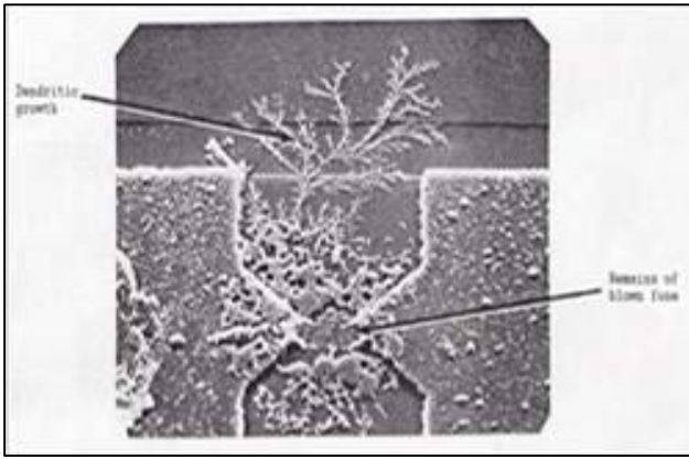
Figure 8: A dendrite has grown from the remains of a programmed cell (blown fuse) in a PROM storage device. 14
