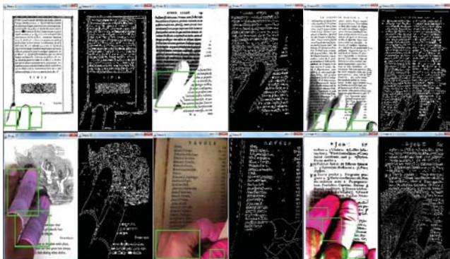
Figure 3: Positive detections of fingers on scans with associated edges where suspected areas are marked by green rectangles.
