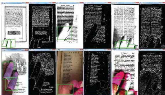
Fig 3. Positive detections of fingers on scans with associated edges where suspected areas are marked by green rectangles.
