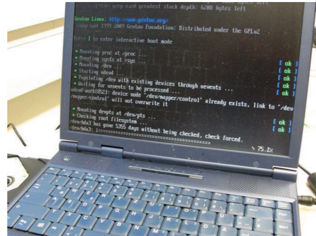
Figure 4. Why you should do disk imaging before anything else: “/dev/hda3 has gone 5355 days without being checked, check forced”.
